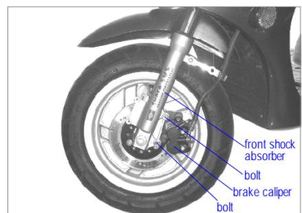
\* Do not pull brake lever when brake caliper is removed so as to prevent jamming of brake block.
