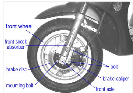
Remove brake disc mounting bolts.
