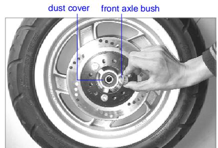
Turn bearing inner race to inspect sliding.
