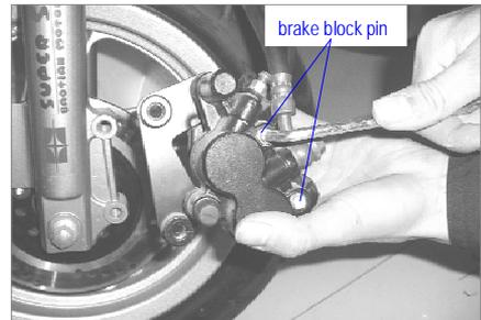
Remove two pieces of brake block pins by means of a hexagon wrench.
