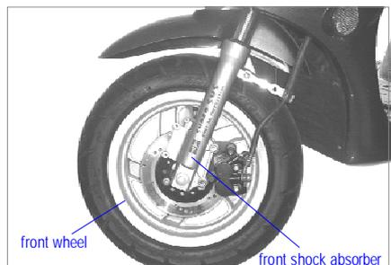
Remove 4 pieces of bolts on the upper part of front shock absorber.
