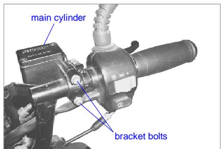
Remove brake light switch and brake lever.
